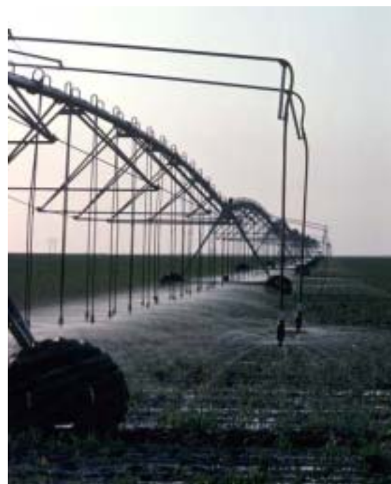
A CENTER PIVOT IRRIGATION SYSTEM WITH DROP TUBES
