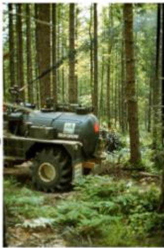
Biosolids forest land application. (EPA photo)
